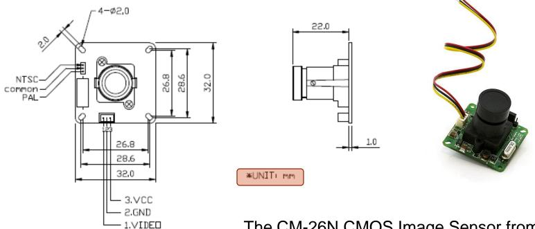
The CM-26N CMOS Image Sensor from Sparkfun Electronics
